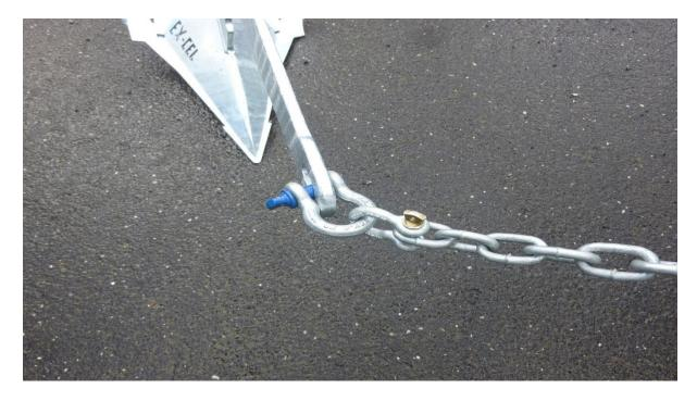
If the bow shackle will not fit through the chain then down size as above, be sure to wire-mouse of the screw pin on the shackles.
